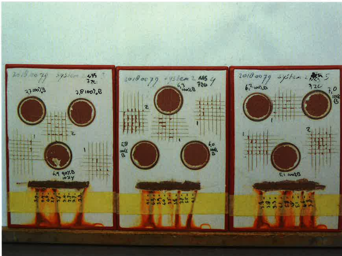
Photo 2: Panels 2.3, 2.4 and 2.5 after 720 hours Neutral Salt Spray test.
