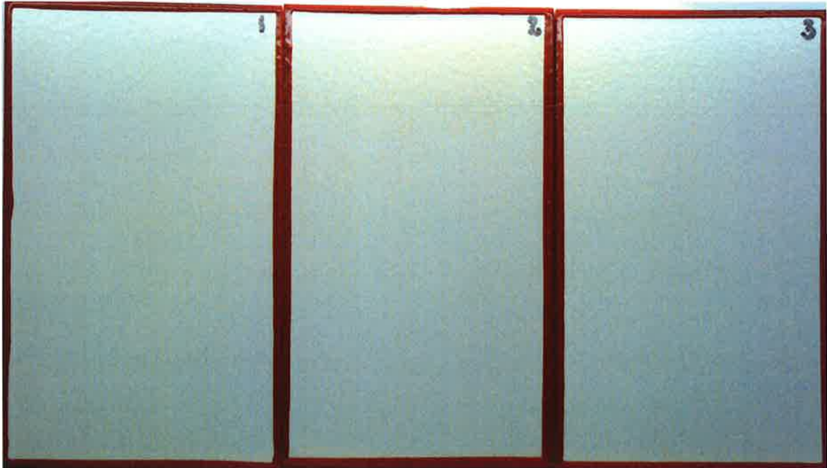
Photo 3: COT sample number 13-06-18/0387, Panels 1, 2 and 3 after 480 hours Water Condensation test.
